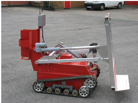
**FIREMOTE FITTED WITH WATERWALL LIFTER**
